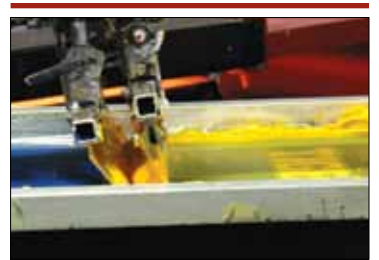
Ink can be applied to a garment by hand or with an automatic screen printing press.
