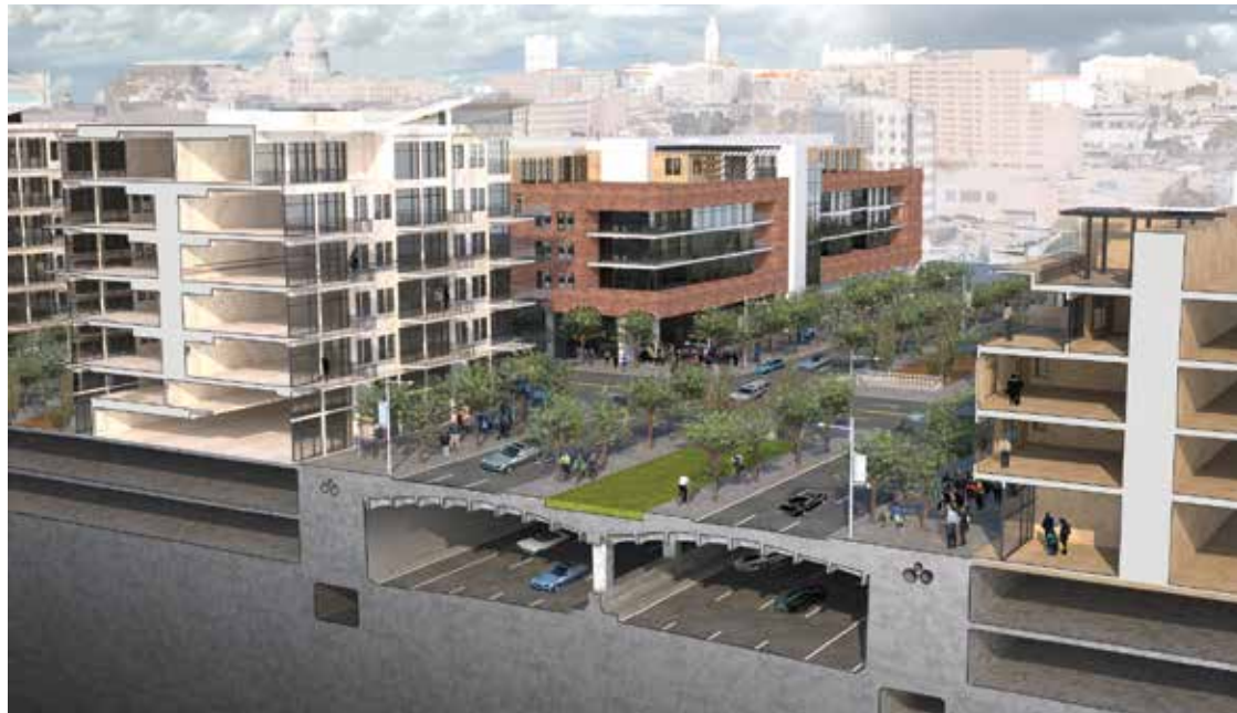
The cut-and-cap proposal would sink I-35 below ground, which would create new developable land through downtown.
