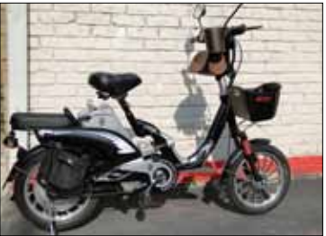
Electric bicycles cost about $1,250, max out at about 20 mph and travel about 30 miles on a single charge. Pedaling can push the range to 50 miles.
